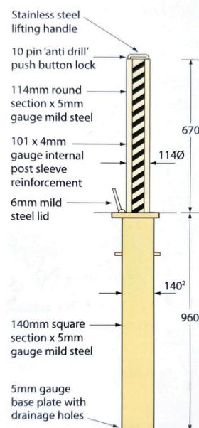
**Rhino-Bollard Phantom** poses a high safety risk. Available in traffic blue, black, slate gray, and red. Height 670 mm, diameter 114 mm. Shaft length 960 mm. Weight 55 kg. Operating weight 17 kg
