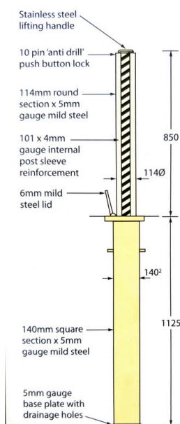
**Rhino-Bollard Cullian for high-risk safety. Available in most common RAL colors. Height 850 mm. Diameter 114 mm. Shaft length 1125 mm. Weight 66 kg. Operating weight 7 kg. With gas spring.**
