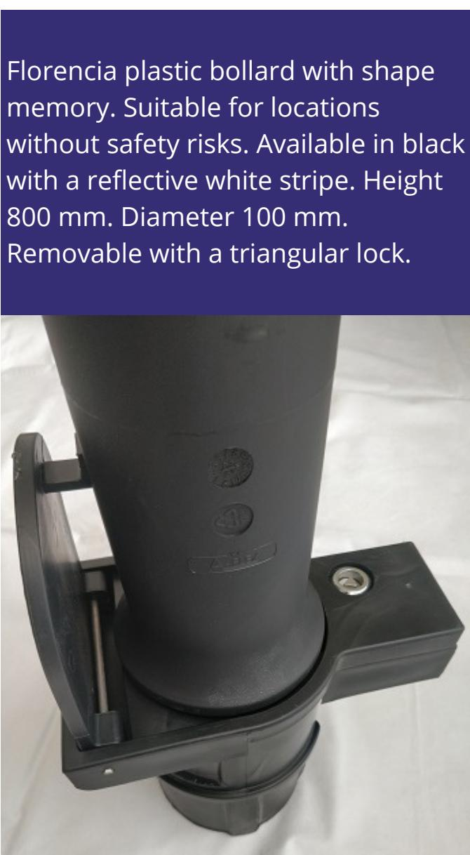
Florencia plastic bollard with shape memory. Suitable for locations without safety risks. Available in black with a reflective white stripe. Height 800 mm. Diameter 100 mm. Removable with a triangular lock.
