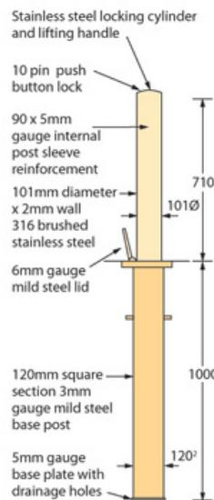
**Rhino-Bollard Corniche for a moderate safety risk. Available in brushed and clear-coated 316L stainless steel. Height 710 mm, diameter 101 mm. Shaft length 1000 mm. Weight 40 kg. Operating weight 17 kg.**
